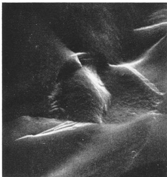
Figure 7 Unetched fractured surface of glass-ceramic heat-treated at 1000^{\circ}\text{C} . The glassy areas (smooth) may be differentiated from those which were crystalline (coarse) at fracture, \times 2800 .
